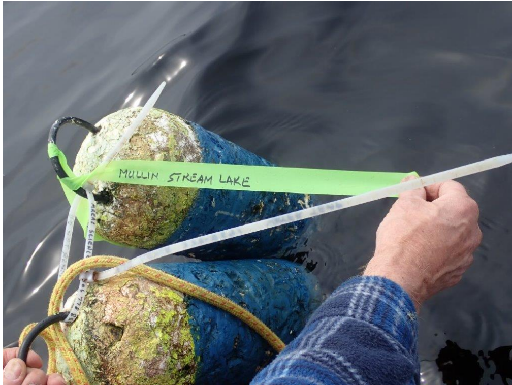
Figure 6: Deploying Water Temp. Profile Logger Line – Mullin Stream Lake May 12, 2023
